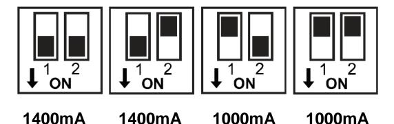
The driver will be shipped out of factory with both switches set to ON (1400mA).
